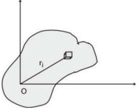
Let us consider the body as being made up of a large number of point masses and one such mass be mi  $\tau = \sum \tau_i = \sum_{i} r_i \times m_i \, g = (\sum_{i} m_i r_i) \times g \quad \text{Q } g \text{ is constant}$
